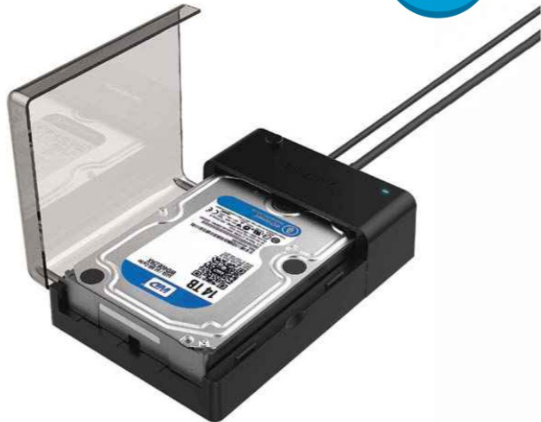
Transform an internal hard drive into an external one with a USB enclosure
